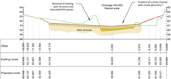
\* To ensure a stable design, sediment sizes through the proto channel section require to be coarse gravel and cobble (with a D50 of 70 mm). If excavated material is not adequate (D50 <70), a minimum of 500mm fill is required.
