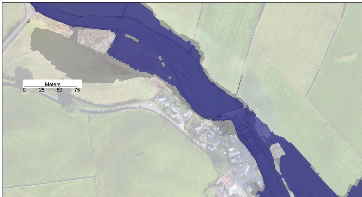
Figure 3.6. 100-year plus 35% climate uplift. Grey area is existing conditions, blue area is design conditions.
